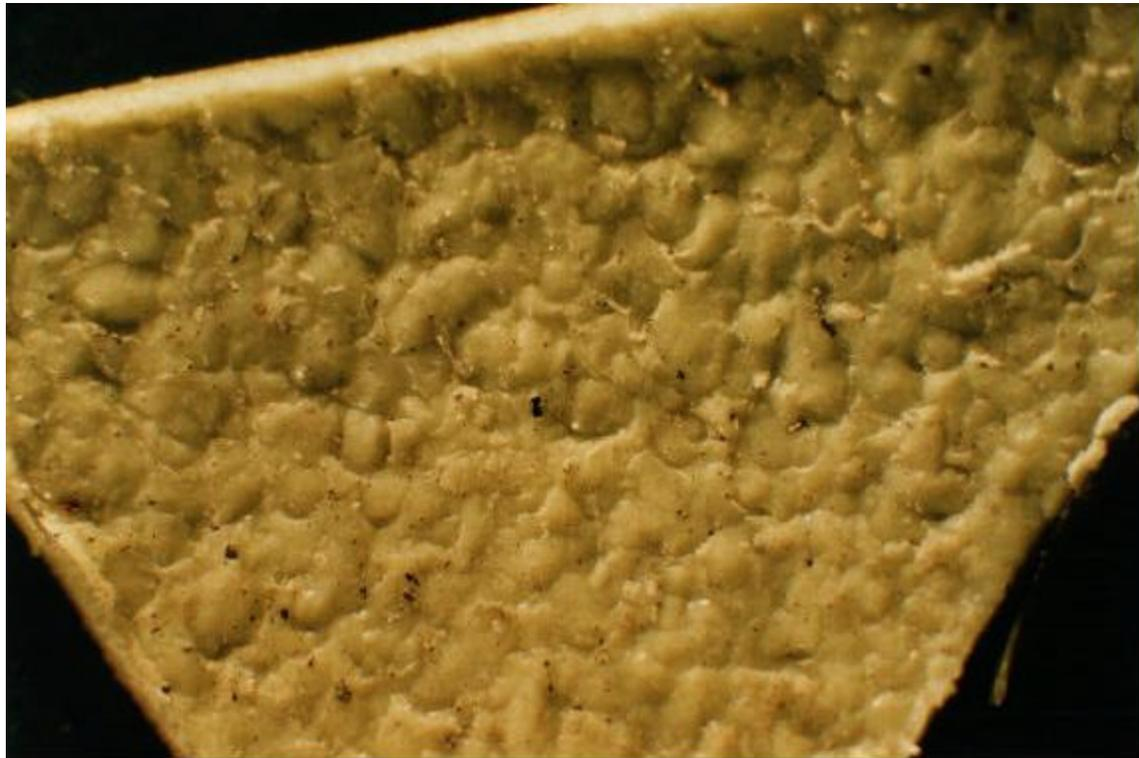
Figure 4.26 Example of Backside Appearance of Coating Removed from Field-extracted ECR Specimens. (~35X)
